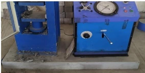
Figure 2: Compression Testing Machine
