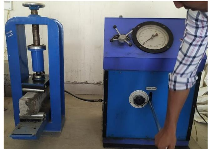
Figure 4: Flexural Testing Machine (Beam specimen under Testing)
