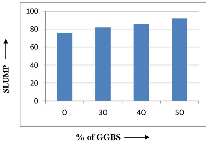
Figure 6: Slump of concrete v/s % of GGBS
