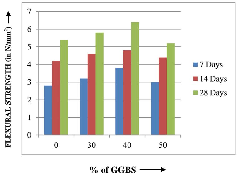
Figure 8: Flexural Strength of concrete v/s % of GGBS
