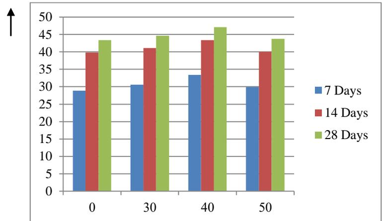
Figure 7: Compressive Strength of concrete v/s % of GGBS
