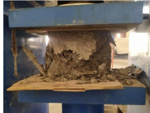
Figure 3: Cube Specimen under Testing
